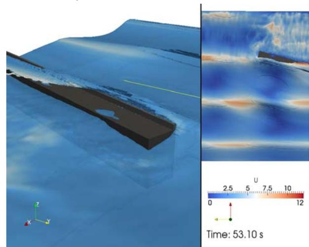
Figure 1 - Regular waves interacting with a vertical breakwater
